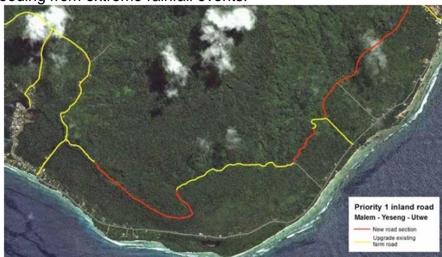
Figure 8 Indicative inland road between Utwe and Malem showing requirements of new and upgraded sections of road
