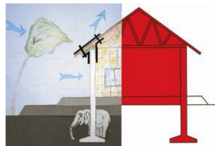
Figure 3-1: Strengthening of rural houses using ties (Source: IFRC BD Shelter Volunteer Training after cyclone Sidr)
