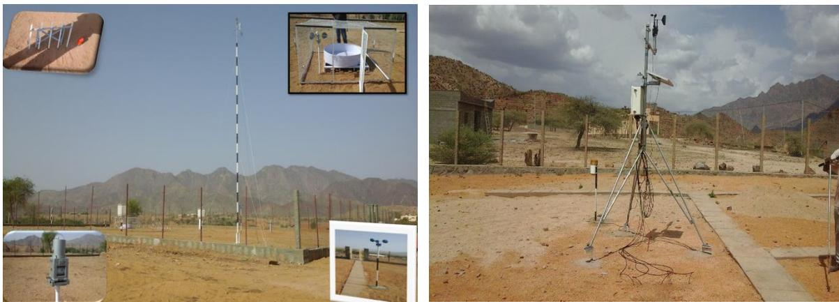
*Figure 12: Class1 Manual weather station at Hamlmalo Agricultural College/Hamelmallo (left) and Class1 Automatic weather station at Habero (right)*
