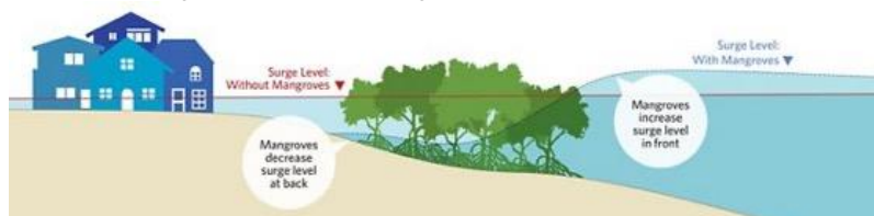
Figure 2827. Storm surge is reduced behind mangroves, helping ease flooding to land and properties. Source: TNC 2018
