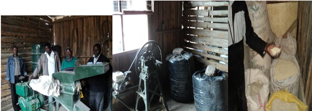
Figure 6: A 20HP chopper grinder motorised chaff cutter and processed silage
