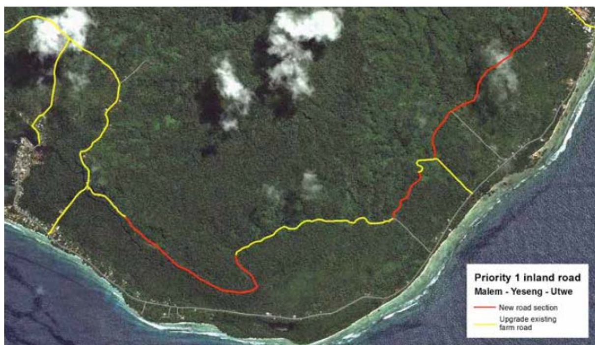
Figure 5: Indicative inland road between Utwe and Malem showing requirements of new and upgraded sections of road
