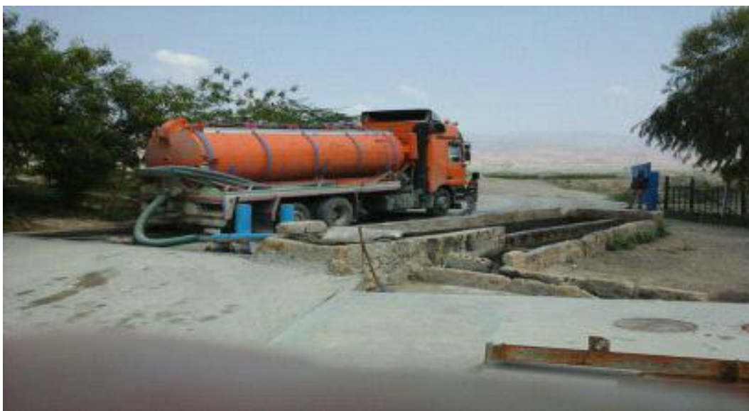
FIGURE 10: SEPTIC TANK EMPTYING TO THE WWTP HEADWORKS
