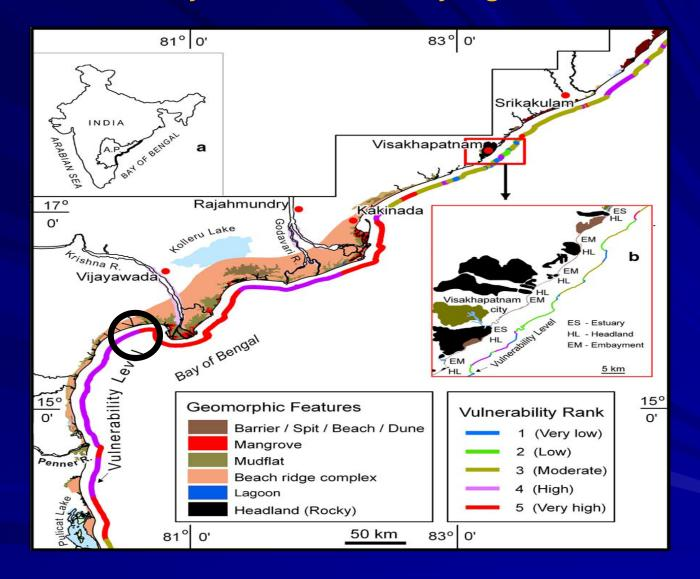
Five physical variables: geomorphology; slope; shoreline change; wave ht; spring tidal level
