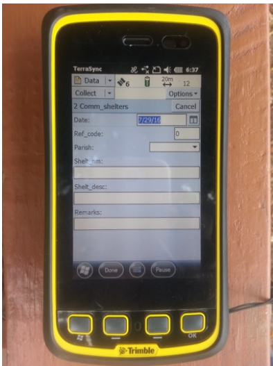
Figure 17. Data dictionary displayed on the Trimble Juno GPS device
