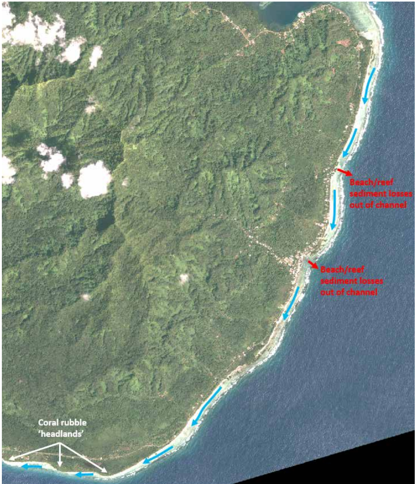
Figure B 11: Key sediment sources, longshore transport processes, and sediment losses along the Malem shoreline.
