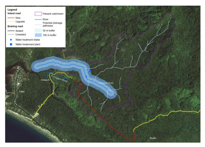
Figure 17 Kuplu Wan road alignment and buffer zones from the Palusrik River.
