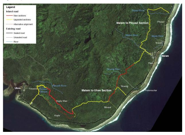
Figure 12: Alignment of inland road between Utwe and Malem. The sections in yellow require upgrading and widening of existing farm roads. The sections in red are new sections of road.
