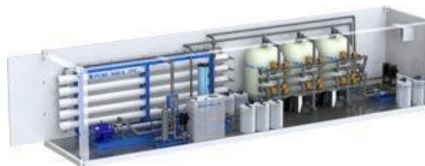
Figure 3: Containerized reverse osmosis desalination system
