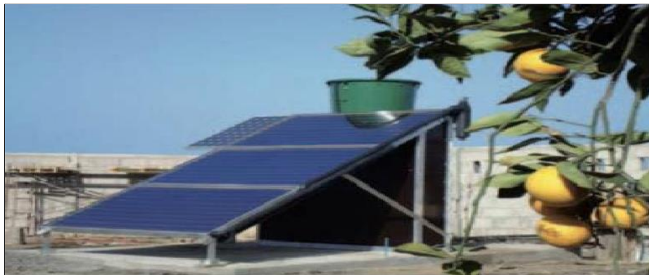
Figure 4: Membrane Distillation installed by SOLARSPRING GMBH
