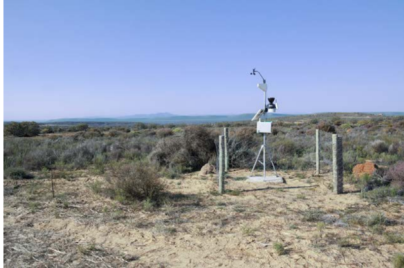
Picture 4: agrometeorological station in a rooibos field as part of the project executed by Heiveld
