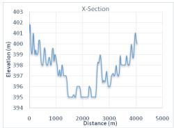
Figure 10 Cross Section of Proposed Location of DAM 1
