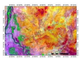
**Plate 2b.** Landsat 8 colour composites image obtained using the OLI band combination 752 in RGB, respectively, decorrelation stretched.
