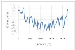
Figure 22 Cross Section of Proposed Location of DAM 7
