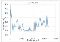
Figure 12 Cross Section of Proposed Location of DAM 2
