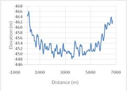
Figure 20 Cross Section of Proposed Location of DAM 6
