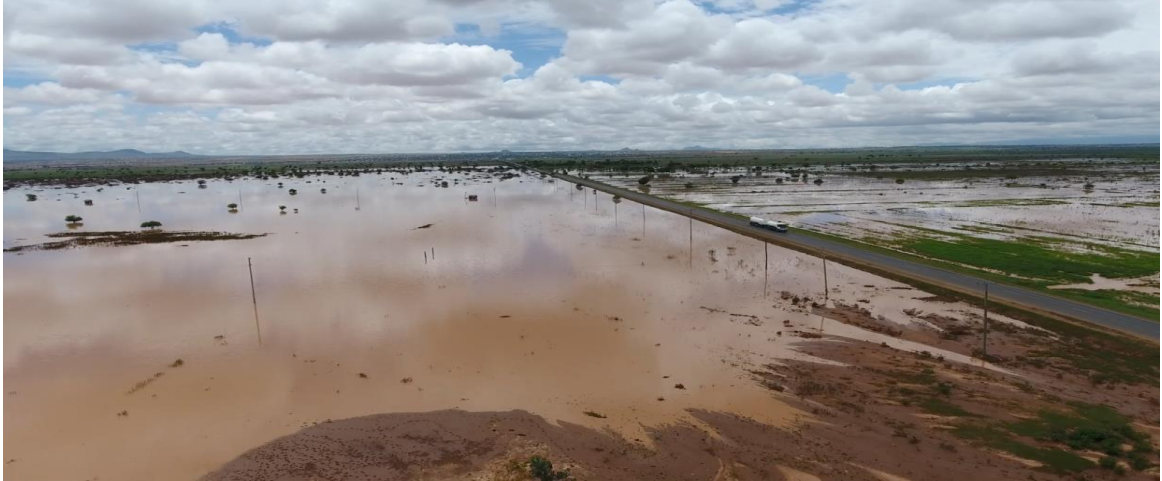
Figure 2: The Mbuga is seasonally flooded. The Dodoma –Dar es Salam road acts as a barrier to drainage.
