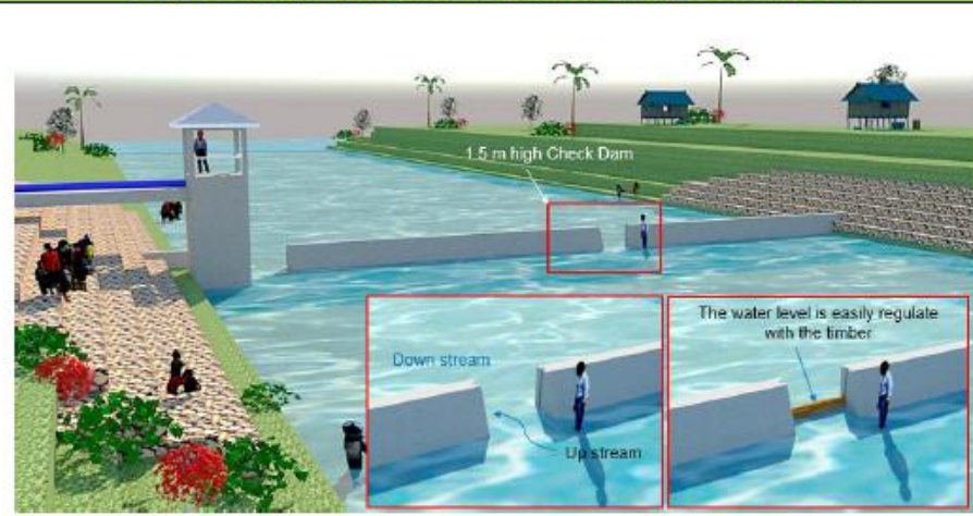
Proposed Raw Water Intake with 1.5 m high Check Dam
