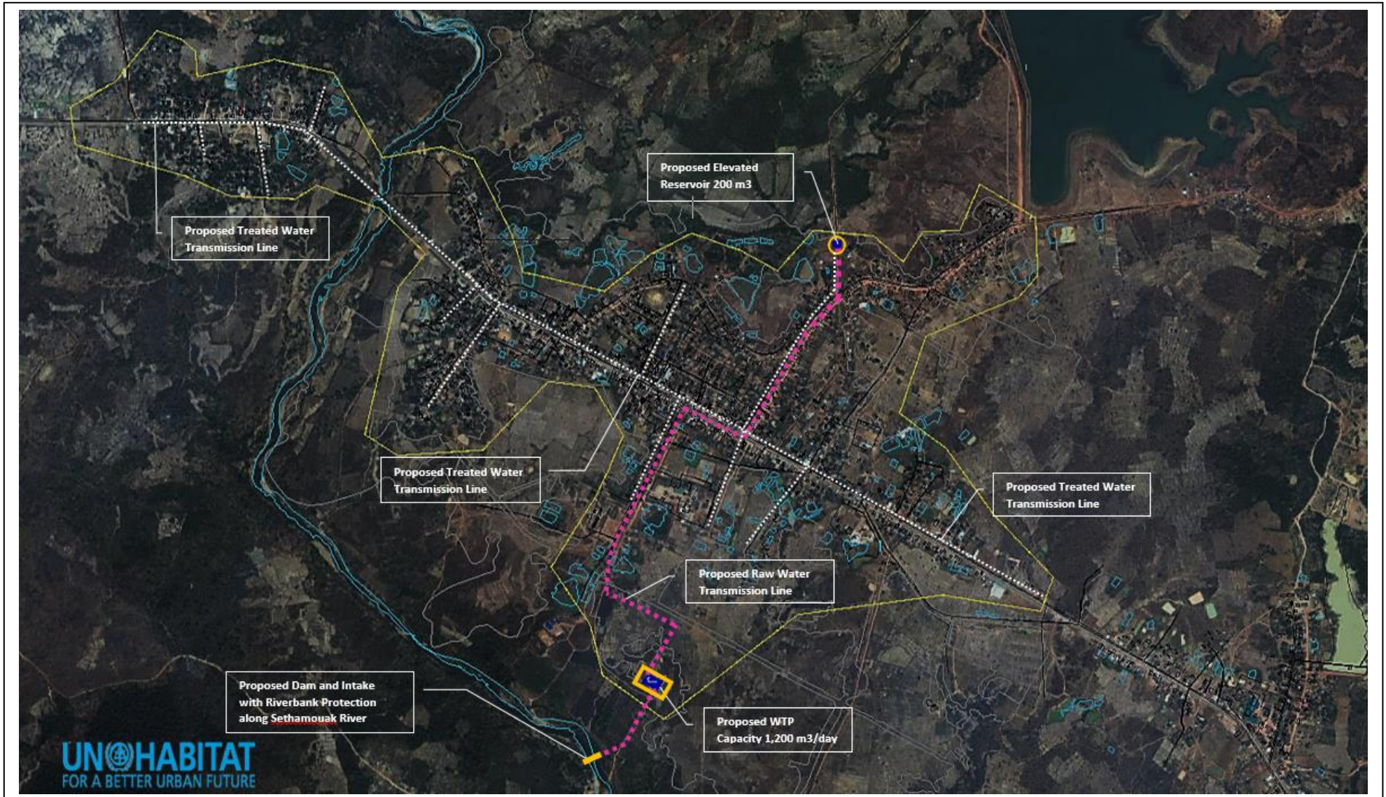
Proposed climate resilient water supply system with capacity of 1,200m 3 /day in Sethamouak Town. Further technical details in Annex 4
