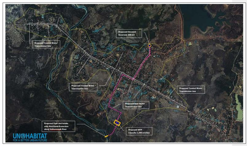
Proposed climate resilient water supply system with capacity of 1,200m3/day in Sethamouak Town. Further technical details in <u>Annex 4</u>
