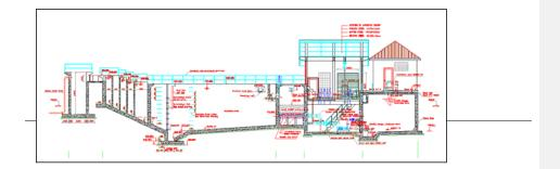
Longitudinal-Section of Water Treatment Plan with capacity of 1,200 m3/day
