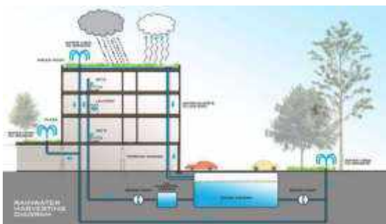
Figure 39: Rainwater harvesting diagram
