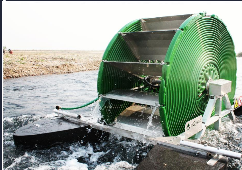
Barsha Pump (Nepal) – irrigation pump powered by streams and rivers to water nearby lands without need for electricity.
