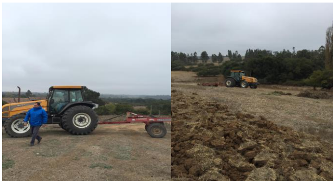
Picture 1: (Left) Subsoiler plough; (Right): Subsoiler plough tool works between 35 to 45 centimeters under the surface, allowing the rupture of compacted soil layers or hardpan.
