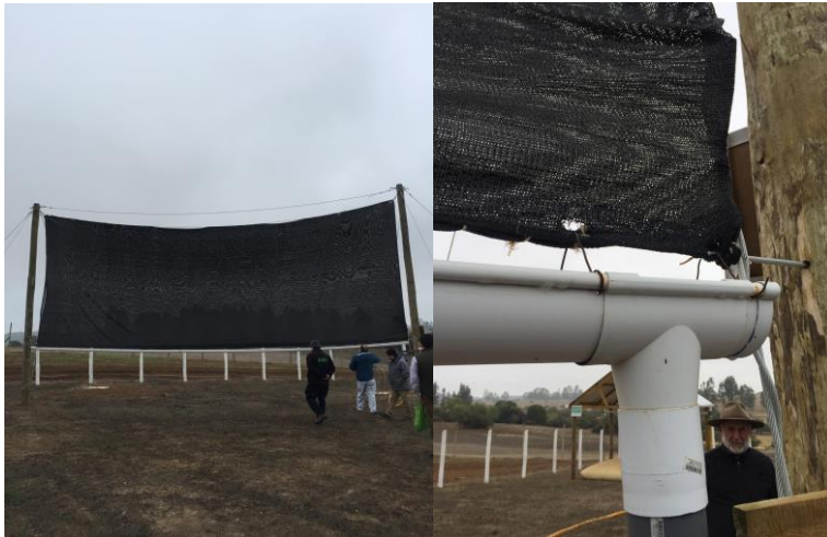
Picture 3: (Left) INIA's "fog catcher" device. (Right) Mist and fog are collected on the large tarp and channeled into water catchment devices.
