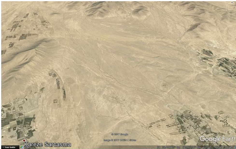
Figure 34 Karez landscape in a perspective GoogleEarth view; the lines of the irrigation tunnels leading from the foothills to the villages are well visible.
