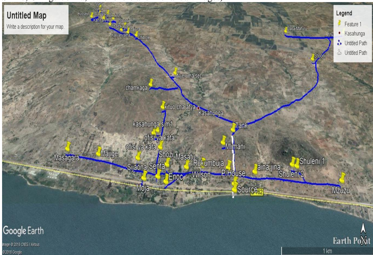
Figure 6: Proposed rehabilitation of water sources and pump house at Kasahunga, Neruma ward to pump water from Lake Victoria for up-country villages (Haruzale, Kemkombyo/Neruma, Chamakapo, Nyamitwebili and Namibu villages)
