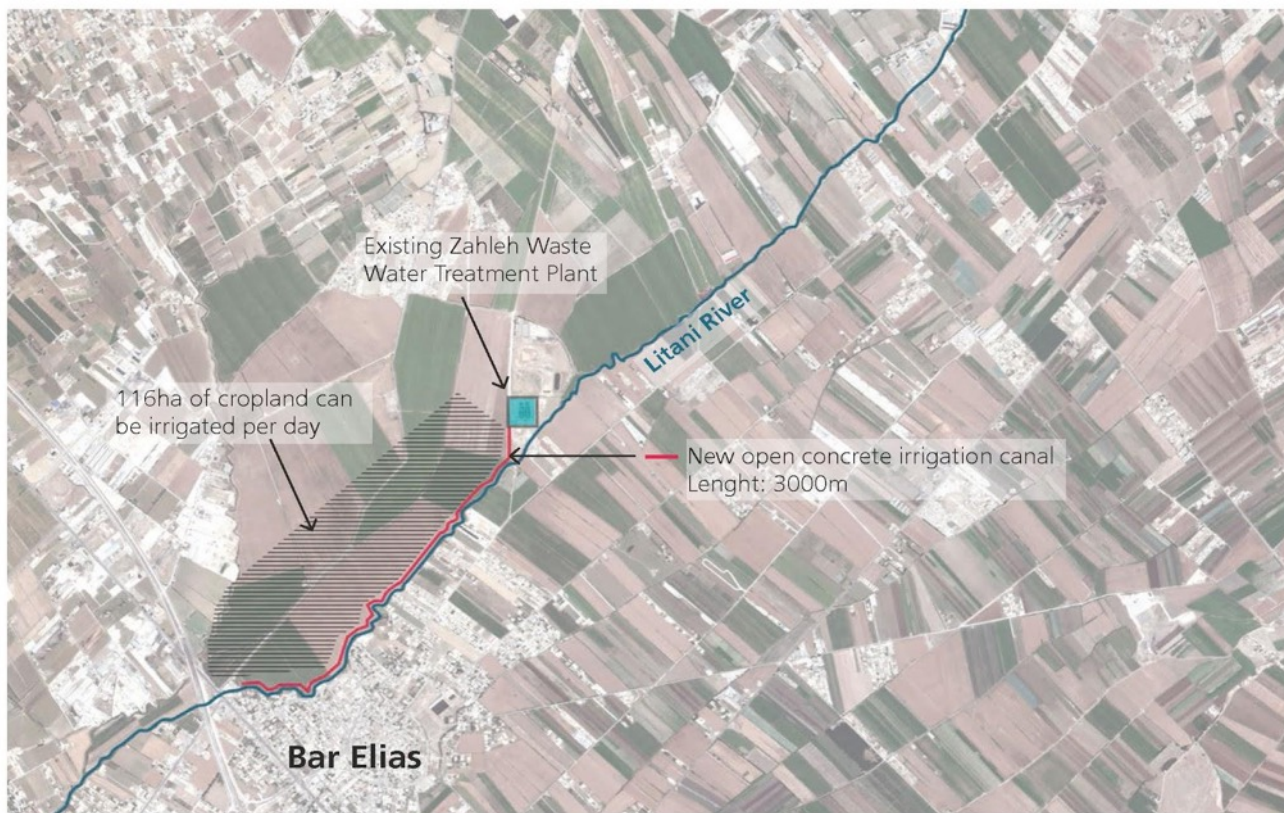
Figure 19: Map showing the reuse of the Zahle Wastewater Treatment Plant (ZWWTP) effluent for irrigation through the installment of a new open concrete irrigation canal
