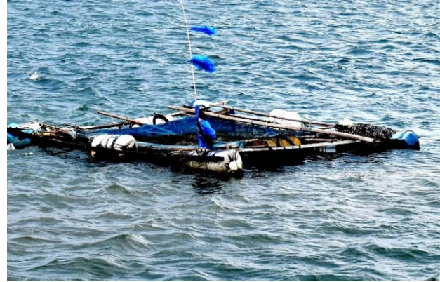
Traditional FADs with wood / bamboo and used drums material
