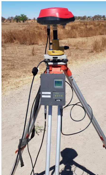
Real-Time Kinematics (RTK) instrument used in survey and topographic survey and design of the catchments for water harvesting
