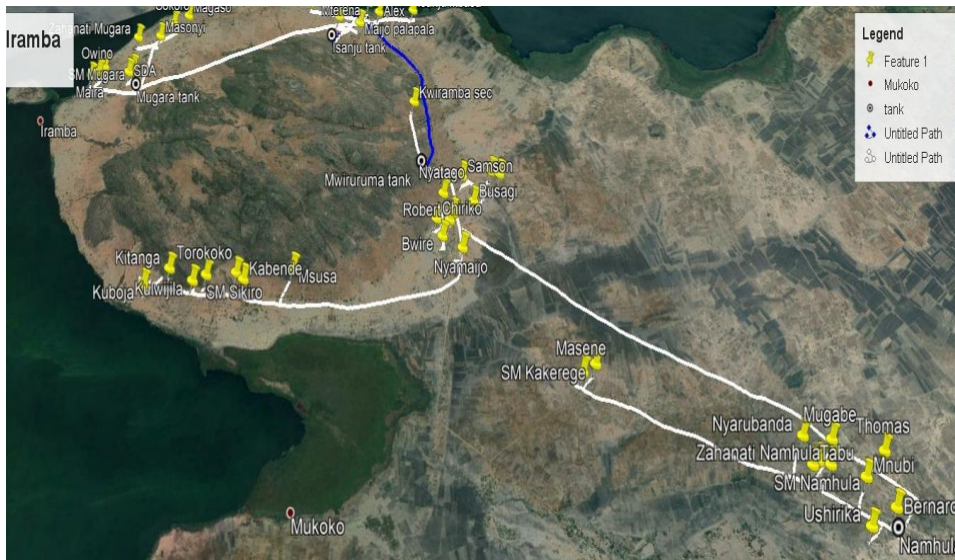
Figure 105: Proposed rehabilitation of water sources and pump house at Isanju, Iramba ward to pump water from Lake Victoria for up-country villages (Namhura, Mwiruruma, Mumagama, Sikiro, Chingulubhila, Karukekere and Mukanda villages)
