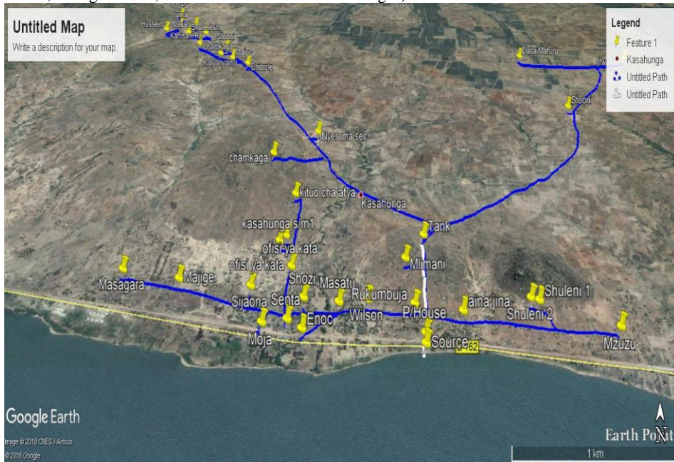
Figure 116: Proposed rehabilitation of water sources and pump house at Kasahunga, Neruma ward to pump water from Lake Victoria for up-country villages (Haruzale, Kemkombyo/Neruma, Chamakapo, Nyamitwebili and Namibu villages)
