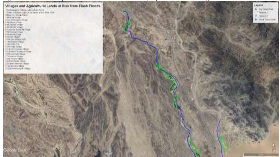
Figure 59 Detailed maps of areas at risk of floods and proposed locations of gabions
