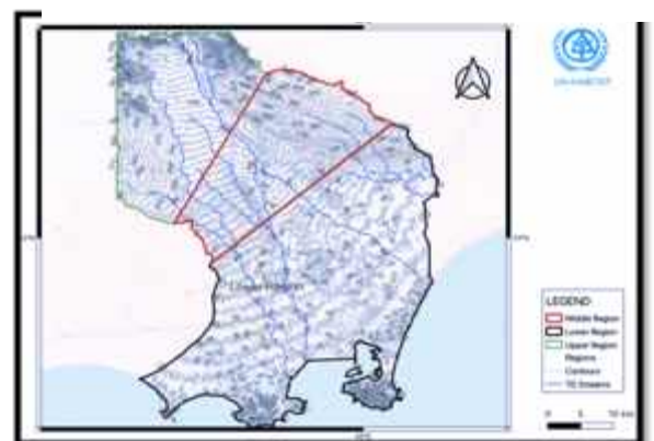
Figure 55 Tuban Delta regions with contours and streams delineated, UN-Habitat (2023) Hydrology report for the Tuban Delta
