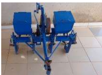
SRI Direct seeder developed by SOCAFON in Mali
