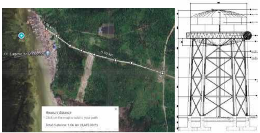
Figure 12. Distance from the water reservoir to barangay Tongmageng and the proposed design of an elevated Water Reservoir with a height of 30m.
