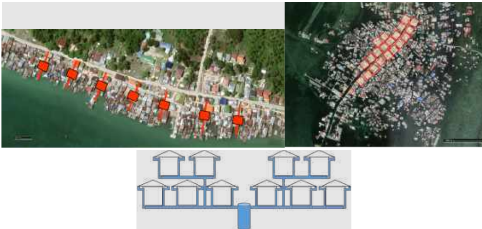
Figure 18. Illustrative example of communal rainwater harvesting clusters
