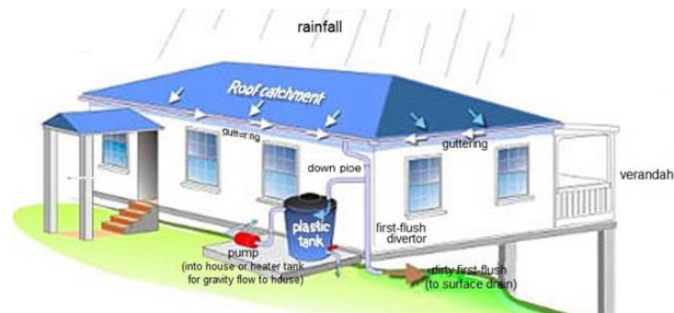
Figure 2049. System designed by GWP-NIHERST, to be adapted by the project to also mitigate floods.
