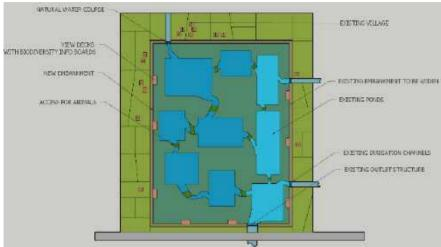
Figure 6 Schematic general arrangement plan (illustrative only)
