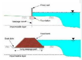
Figure 3 Typical elements of a permanent flood protection system <sup>5</sup>
