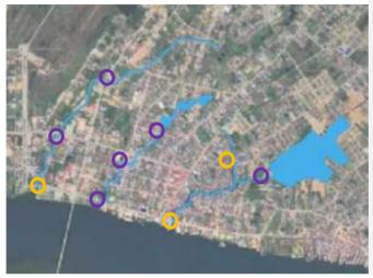
Figure 14 Initial Recommendation for Location of Trashbooms
