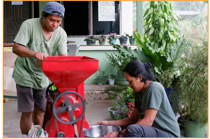
Zeth Toranda (left), also known as Pong Cia, a member of the Forest Farmers Group in Bokin Village together with Irfan, a KAPABEL Field Officer, processed coffee from parchment to green bean by using a huller. (Photo by Kemitraan)
