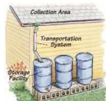
Figure 9 Conceptual diagram for rainwater harvesting system
