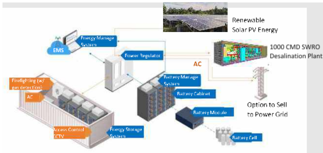
Figure 9. Illustrative diagram of a solar PV energy system attached to the SWRO desalination plant
