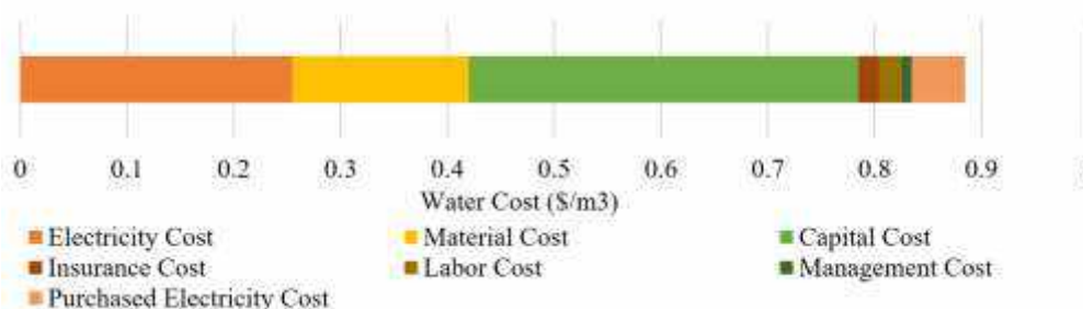
Figure 13. Average cost breakdown (Levelized Cost of Water) for large reverse osmosis desalination plants
