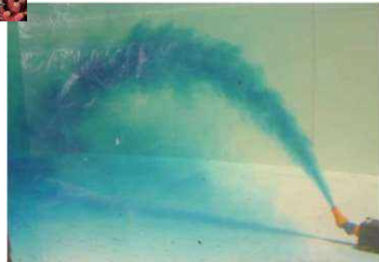
Brine being discharged through a Jet
