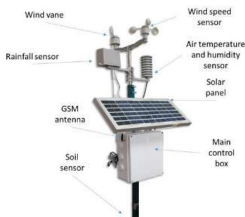
Figure 4. Scheme of an agro-meteorological station (Source: UNDP 2021 )
