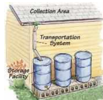
Figure 9 Conceptual diagram for rainwater harvesting system
