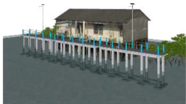
Figure 4 Perspective for proposed raised pathway design.
