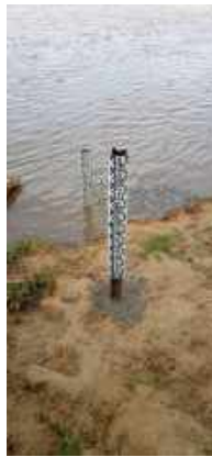
Water level gauge
