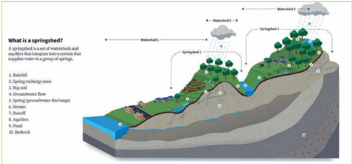
Figure 4: Schematic diagram of a springshed
