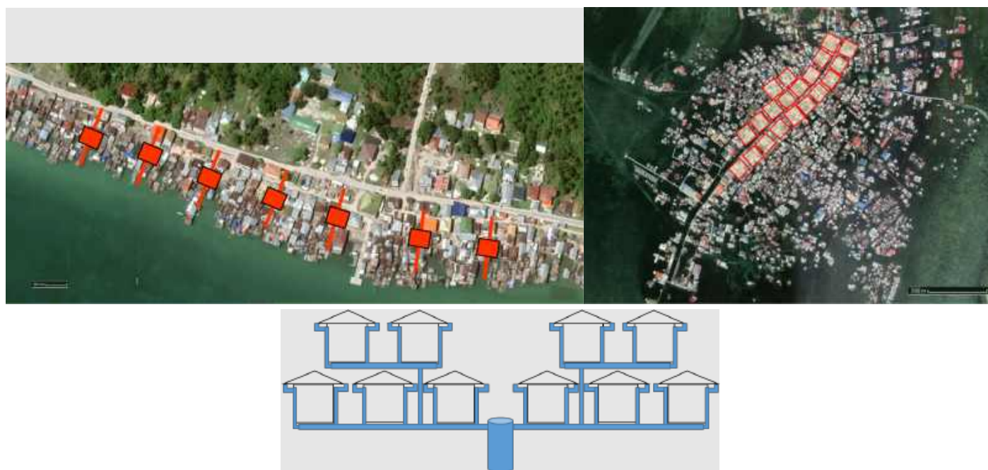
Figure 18. Illustrative example of communal rainwater harvesting clusters
