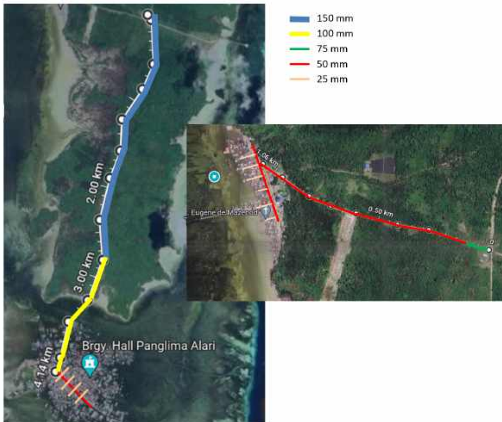
Figure 15. Pipeline layout for Sitangkai proper (Left) and Tongmageng (right) using transmission lines 150, 100, 75, and 50 mm pipes. Lateral pipes using 25 mm diameter.
