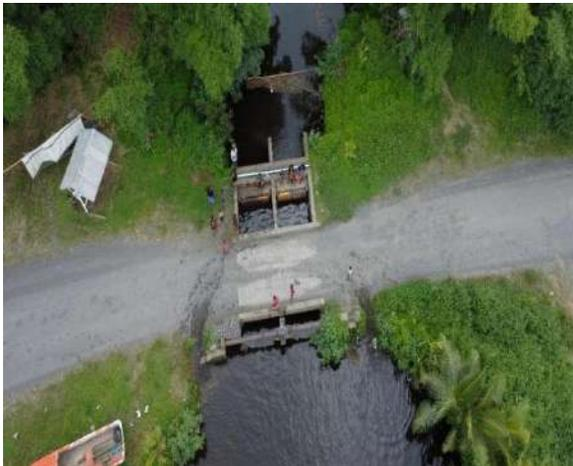
Figure 12 Vuci village and the existing 2-barrel flood gate which needs repair through replacement of steel gates.
