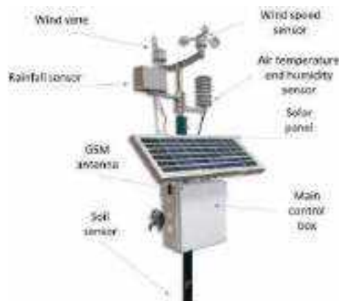
Figure 4. Scheme of an agro-meteorological station (Source: UNDP 2021 )
