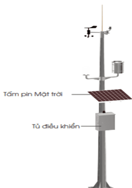
Figure 9. Smart rainfall monitoring station
