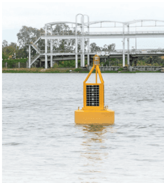
Figure 10. Floating water level and water quality/salinity monitoring
