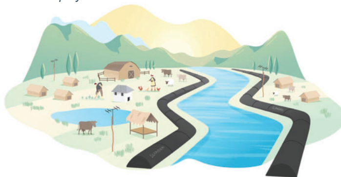
Figure 8 Mobile flood barrier deployed
