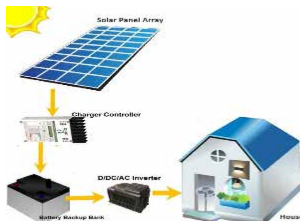
Figure 6. Schematic Diagram of Off-grid Solar Power System
