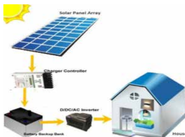
Figure 5. Schematic Diagram of Off-grid Solar Power System
