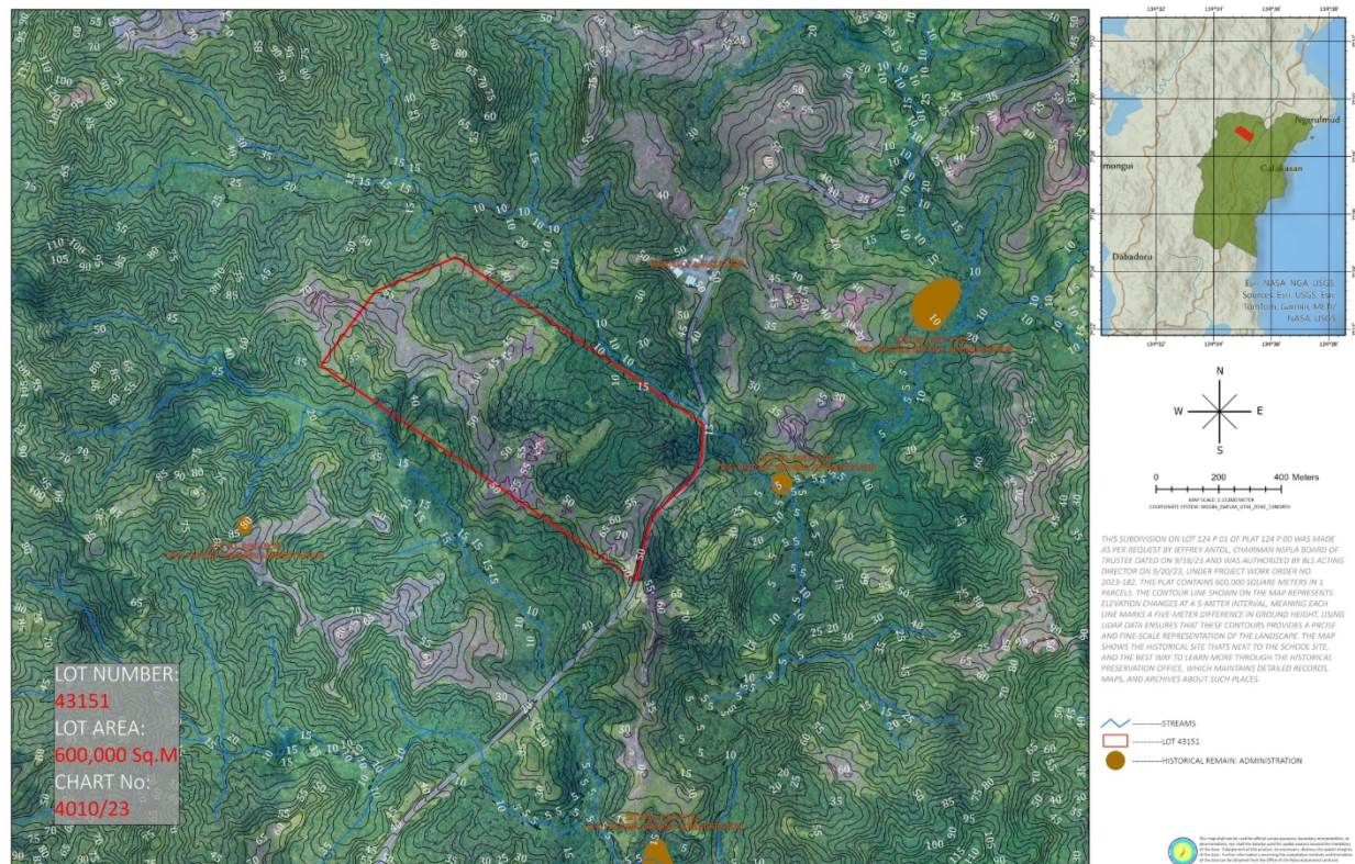
Figure 11: LiDAR 5 m contour map of the proposed Desbedall school site (Lot 43151; about 60 ha), Ngchesar State. The site occupies higher inland ground at roughly 35 to 65 m, well above the coastal hazard zone, and drains to interior streams. Nearby historical-remains sites are marked, and an archaeological survey of the site is planned. Source: 2025 LiDAR, PALARIS (Chart No. 4010/23).
