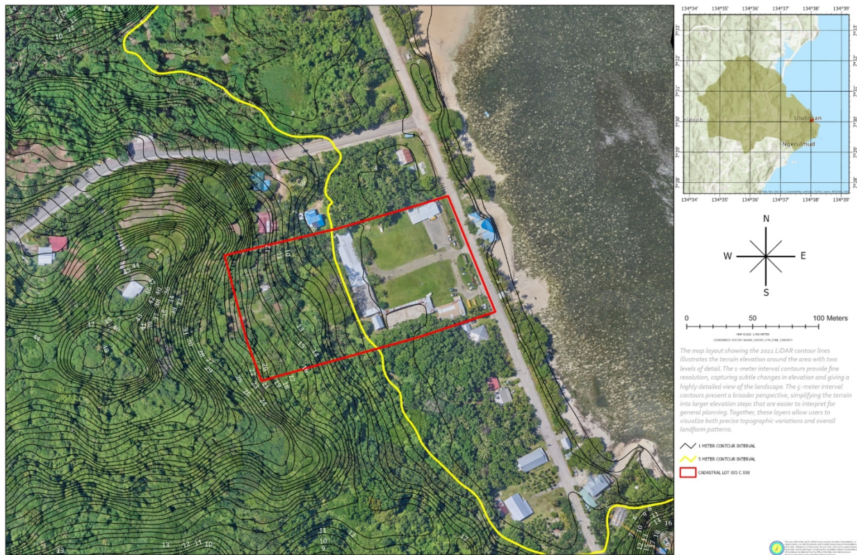
Figure 5: LiDAR contour map of the existing Melekeok Elementary School site (Cadastral Lot 005 C 008), showing the 1 m and 5 m elevation contours. The school grounds sit on the low coastal terrace below the 5 m contour, just behind the shoreline. Source: 2021 LiDAR, Office of the Palau Automated Land and Resource Information System (PALARIS).
