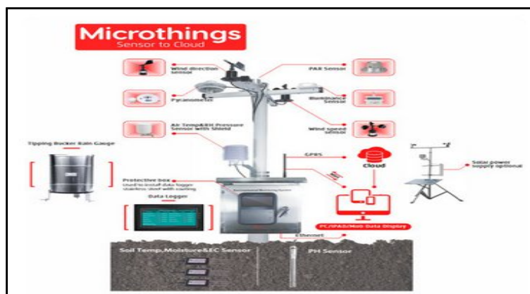
Figure. 8 Automatic Weather Station (AWS) operating system
